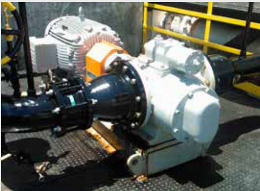
Cargo Pump Fuel Oil 528 gpm / 120 m 3 /h 167 psi / 11.5 bar
